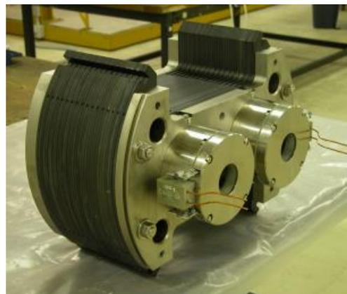
**MQT coils inserted in the yoke**
