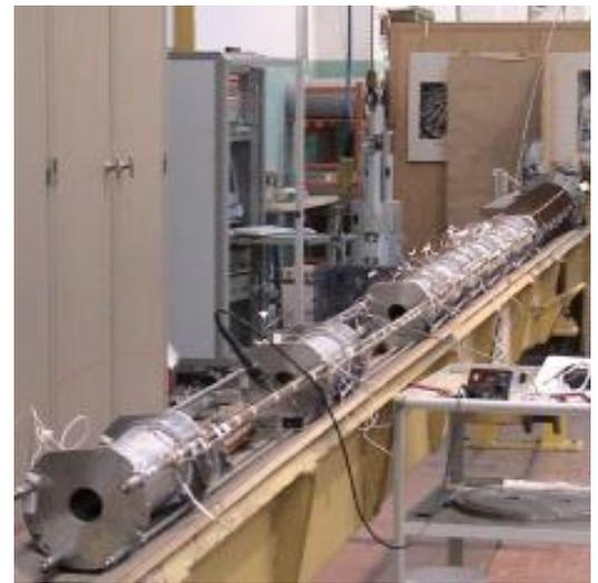
**MQTs cold test in HERA cryostat**
